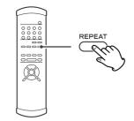
Use the REPEAT button to select the repeat mode for playback. Repeated presses of the REPEAT button cycle between the following options:
